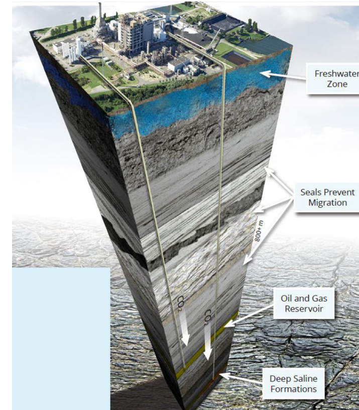
Figure 1. Block diagram illustrating the relationship between deep saline formations for CO2 storage, shallow freshwater aquifers and surface facilities (PCOR Partnership Atlas, Energy & Environmental Research Centre, 2021)
